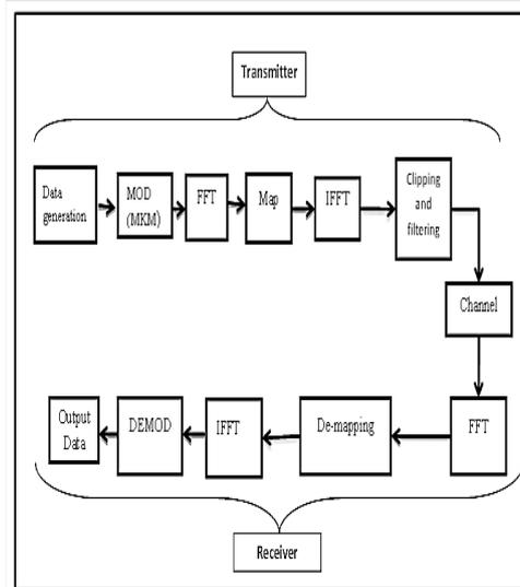
**Fig.1.** Transmitter and receiver of System Model
